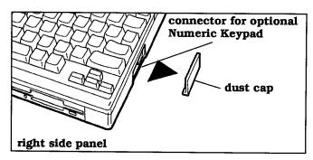
A dust cap is provided for the numeric keypad connector. Remove and store this cap in a safe place while the connector is in use.
